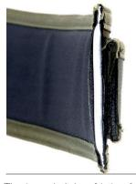
The inner belt has friction fabric on the inside, then foam, then hard plastic, then fabric and finally hook Velcro. The outer belt is made with loop Velcro on the inside, then hard plastic, and webbing on the outside.
