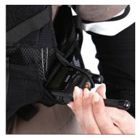
The radio is secured with an elastic string that makes it possible to pull up the radio and change the channel.
